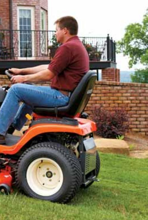
All GR mower decks are constructed of durable 10-gauge steel and designed with a 5-inch deep shell to assure professional and lasting results. And with an easy to reach cutting height adjustment dial and hydraulic mower deck lift, your professional results just became easier to manage. For even finer clippings, an optional mulching kit is also available.
