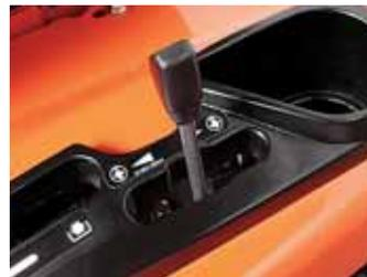
*Hydraulic mower lift lever*
